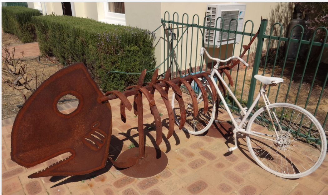
A local metal fabricator has created this very innovative bike parking facility which is located outside the Five Roads Café in Calingiri. 'One-off' installations, as long as they provide the necessary support for the bicycle frame and places for bike locks to be affixed, would be ideal for several situations around Wongan Hills and Ballidu.
