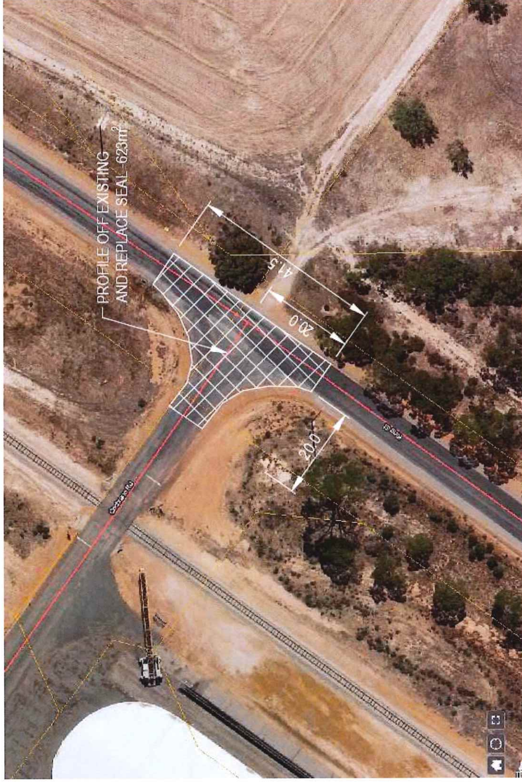
Figure 2: Site Exit at Cochrane Rd & King St intersection – Estimated Area of Seal Defects
